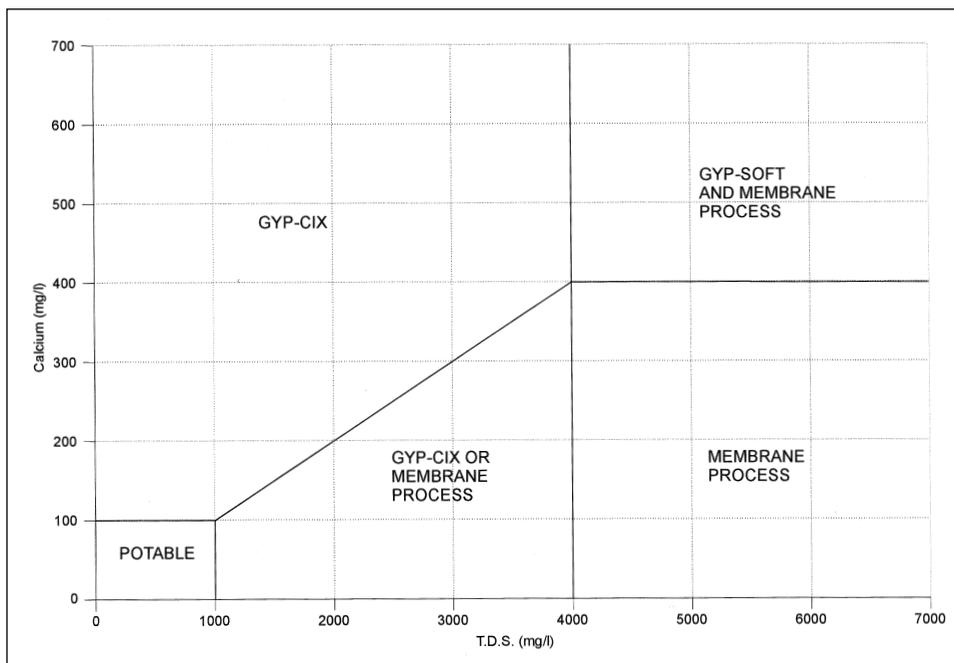
exhausted the resin can be regenerated by the reverse reaction by washing in an acid solution for a cationic resin and sodium hydroxide for an anionic resin. Similar to reverse osmosis, scaling of CaSO<sub>4</sub> is common in conventional circuits. To overcome these problems a modified form of ion exchange has been developed to treat Calcium sulphate waters, for example the GYPCIX (Gypsum Ion Exchange) process offered through Chemeffco of South Africa.
