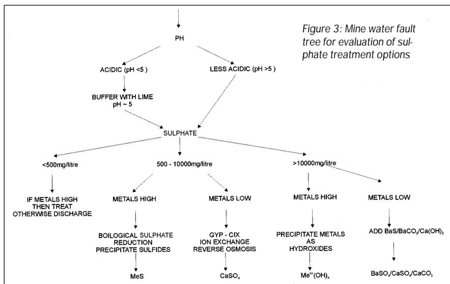
Figure 3: Mine water fault tree for evaluation of sulphate treatment options
