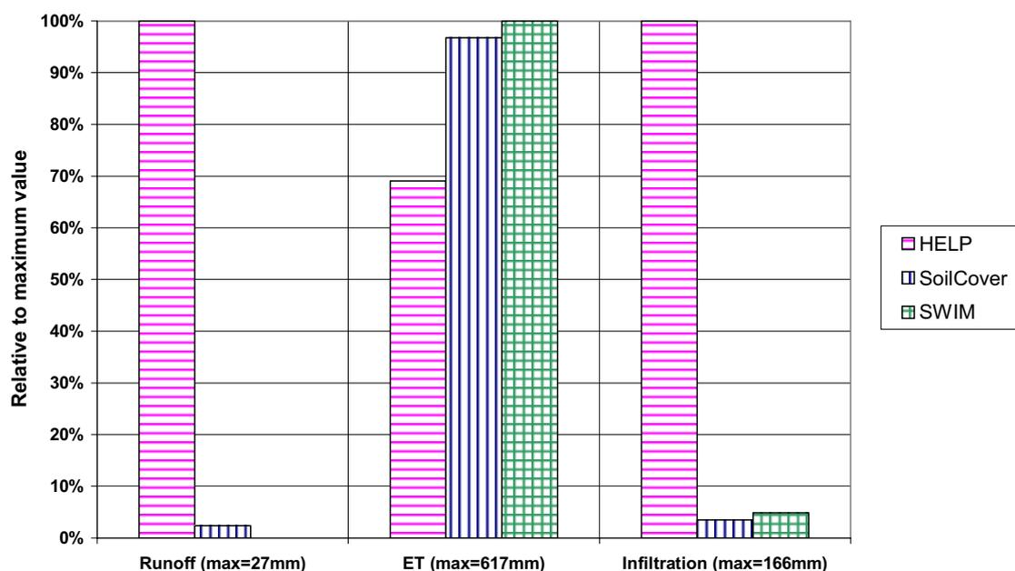
FIG 5 - Water balance comparison, prediction case, average over the five-year period.
