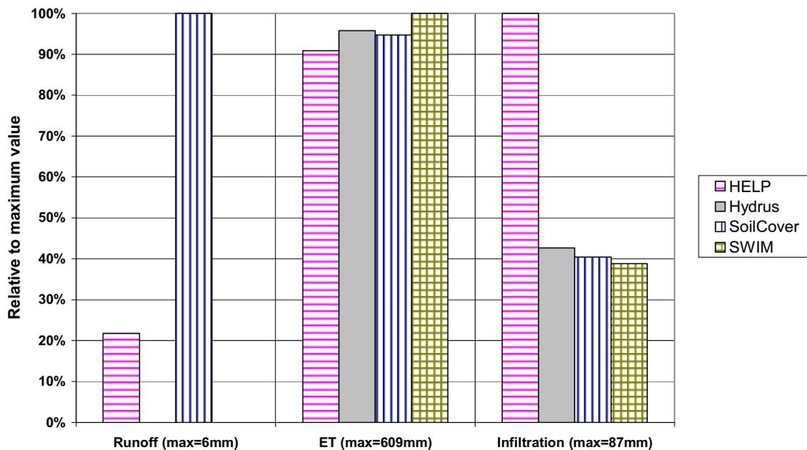
FIG 4 - Water balance comparison, calibration case.
