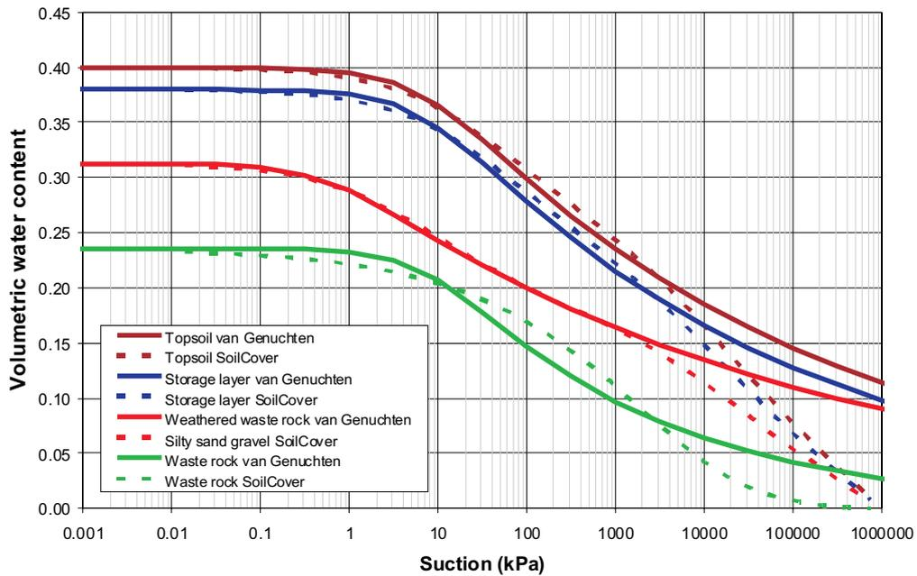
FIG 1 - Fitted soil water characteristic curves.
