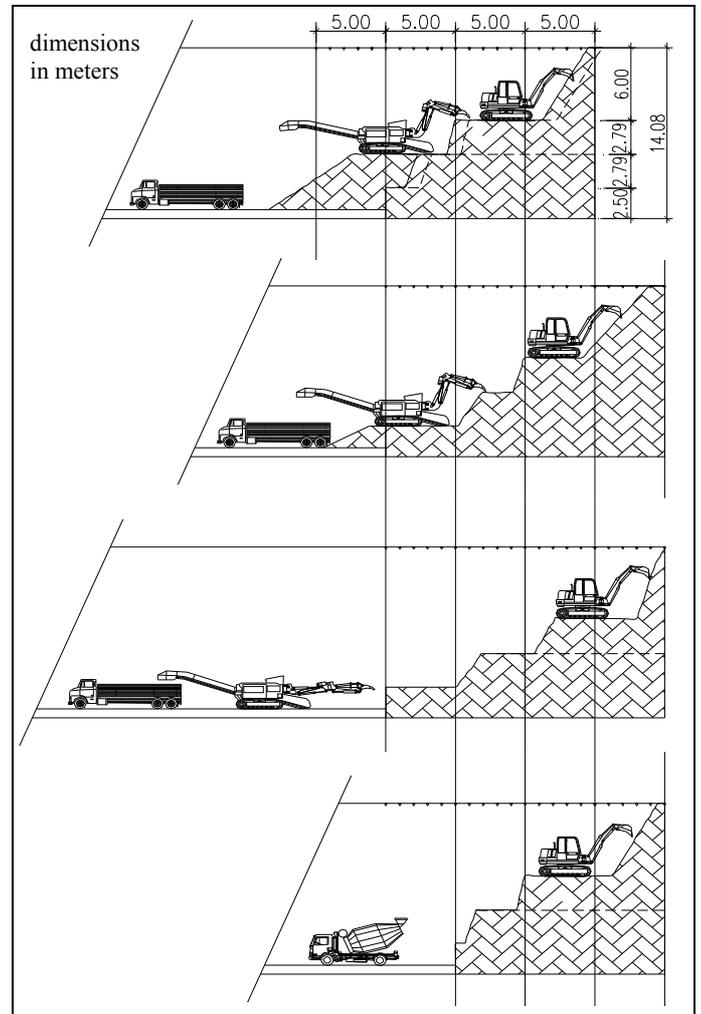
Fig. 11. Construction procedure for Corrientes Station, Line H.
