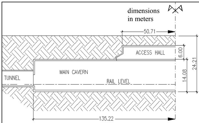
Fig. 10. Longitudinal sketch of Corrientes Station, Line H.
