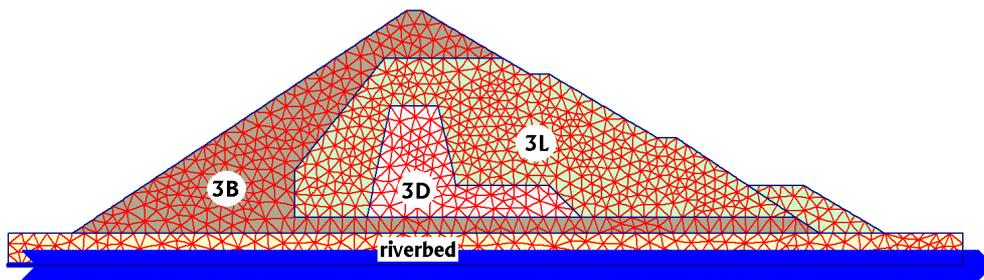
Fig. 4. Mesh and zonification, Los Caracoles Dam.
