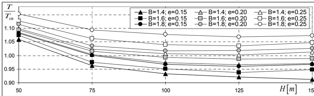
Fig. 3. Numerically computed natural periods  $T$  normalized by  $T_{th}$  given by Eqn (6).
