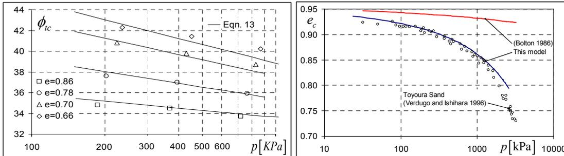
Fig. 2. a: Peak friction angle as a function of mean pressure and void ratio, Toyoura sand. Predicted vs. experimental results. b: critical state line for Toyoura sand. Predicted vs. experimental results.
