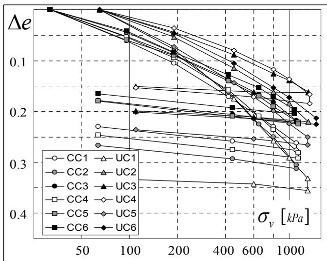
Figure 9. Normalized plot of all 1D compression tests. Scatter is very low for compacted samples and high for undisturbed samples.
