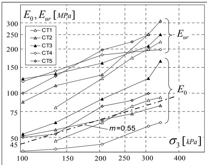
Figure 5.  $E_0$  and  $E_{ur}$  as a function of cell pressure for compacted samples.
