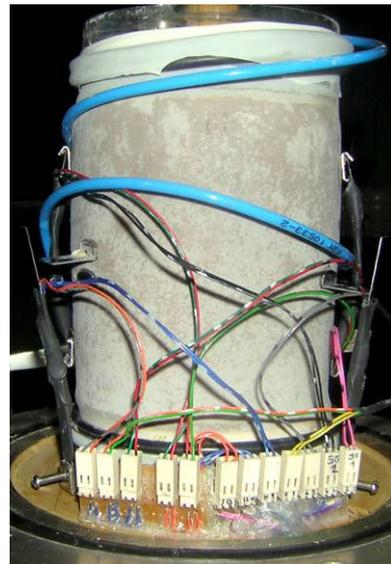
Figure 2. Front view of a sample mounted on the triaxial cell.
