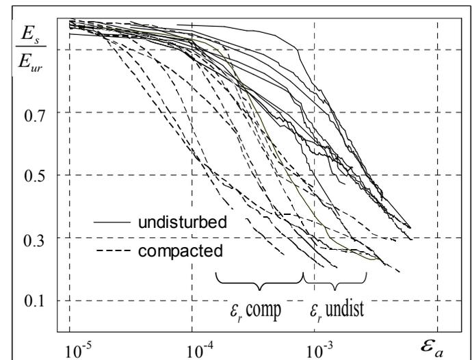
Figure 4. Modulus reduction curves for compacted (dashed lines) and undisturbed (solid lines) samples.
