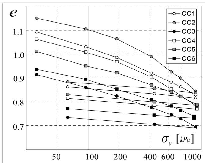
Figure 6. 1D compression of undisturbed samples.
