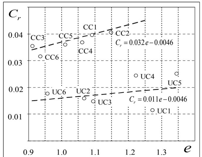
Figure 8. Recompression index of undisturbed and compacted samples as a function of void ratio.
