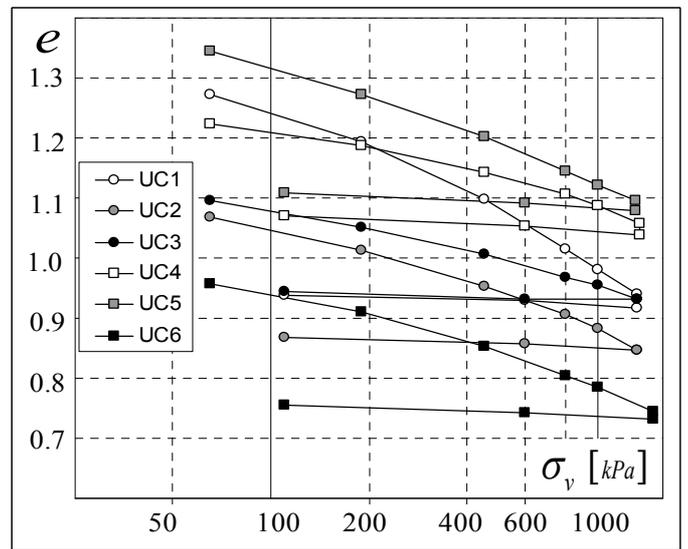
Figure 7. 1D compression of compacted samples.
