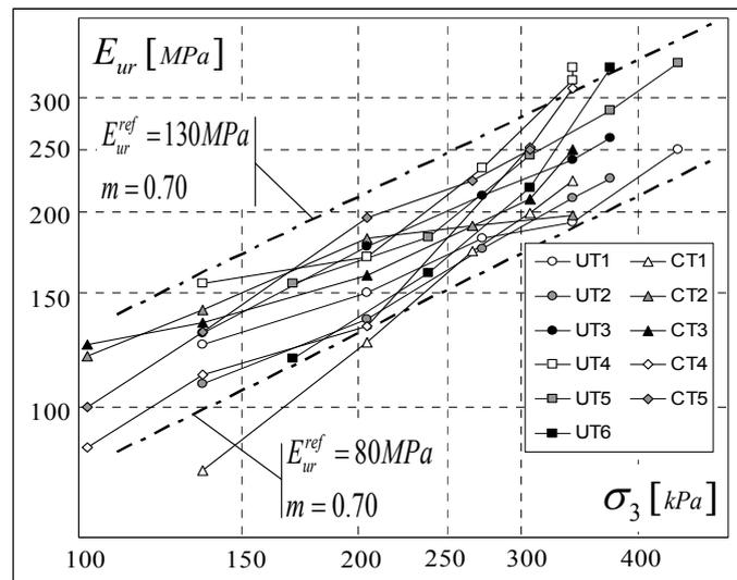
Figure 3. Small-strain Young's modulus dependence on cell pressure. Data from 6 undisturbed and 5 compacted samples.
