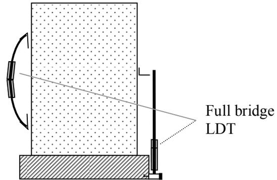
Figure 1. Full bridge axial and radial LDTs.
