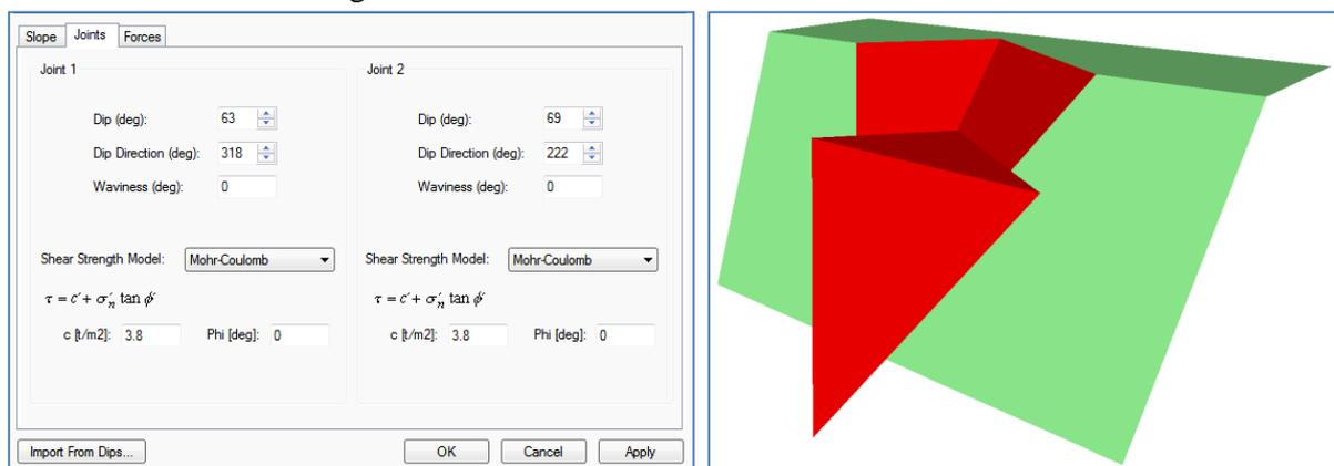
*Figure 2. Menu for definition of joint geometry (Dip, Dip Direction), shear resistance parameters along the joints (Shear Strength Model:  $C'$  and  $\phi'$  - cohesion and friction angle) and type of modelled wedge failure from the bench*
