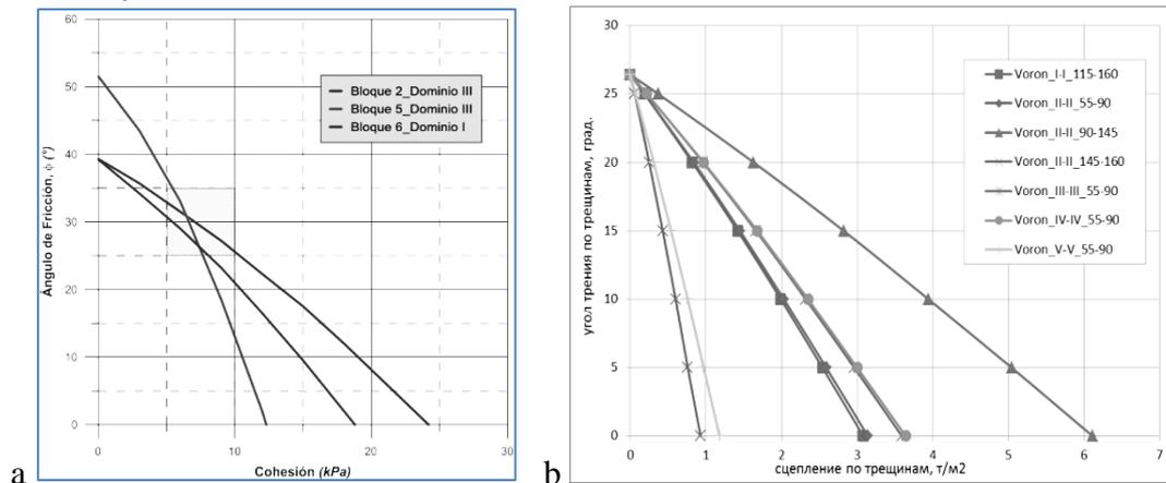
Figure 3. Back analysis of cohesion and friction angle along joints by a set of failures
