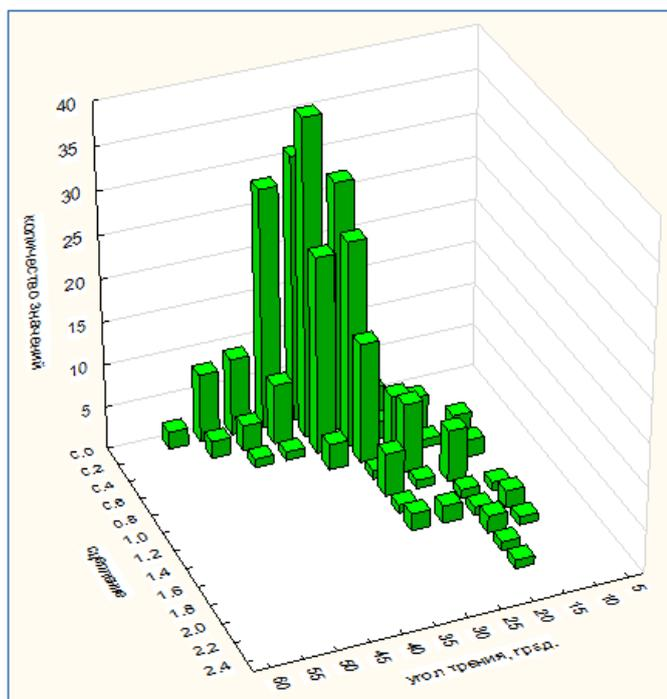
Figure 6. 2D distribution of cohesion and friction angle along joints in the overall set of back-calculated data
