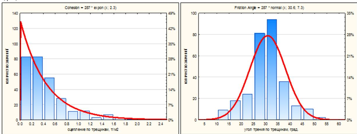
Figure 5. Distribution of cohesion and friction angle along joints for the whole set of analysed data
